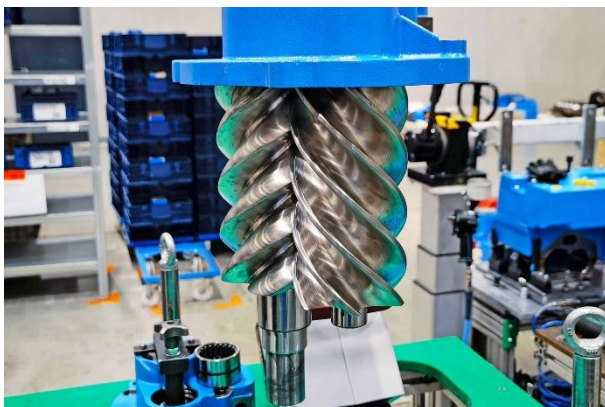
Partially assembled screw compressor assembly, consisting of two rotors and the bearing cover painted blue. © MAPAL
