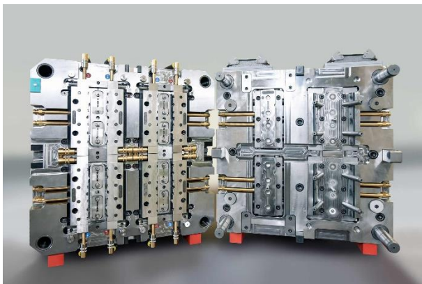
A finished injection mould. © Schülken Form
