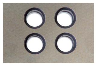
A special CFRP with a "copper mesh" is often used in aircraft construction. Any delamination or fibre protrusion at the bore entrance is avoided when MAPAL tools are used.
