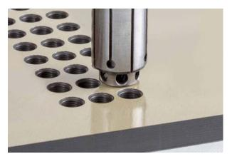
When machining with drill feed units, the tools used must be equipped with additional stabilisation features.
