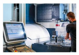
The five-axis machining was carried out on a DMU 80 monoBlock in MAPAL's test centre.
