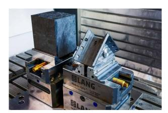
Both clamping set-ups of the part in the working area of the DMU milling machine.
