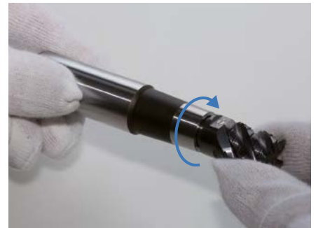
3. Hand tighten the replaceable milling head clockwise into the replaceable head holder. Then clamp the replaceable head holder with the tool in the machine holder.
