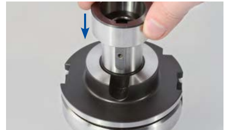
3. Place the first spacer ring on the milling cutter arbor.
