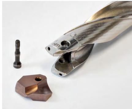
2. Remove the indexable insert from the insert seat.
