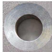
Countersink with extremely unequal spacing
