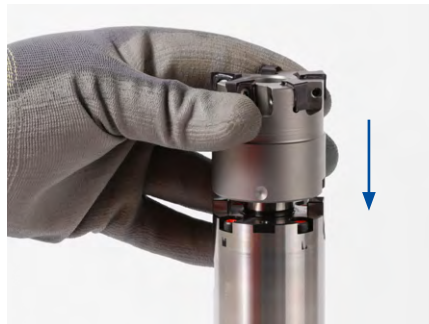
2. Clamp the milling cutter arbor in a changing device.
