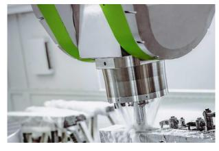
The outer contour is preroughed on the six-axis FZ42 with a VH60 milling head with a NeoMill-Titan. © F. Zimmermann GmbH
