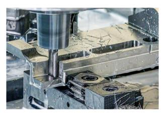
The OptiMill-Tro-Titan finishes the pocket wall. The complete depth is machined in one cut. @MAPAL
