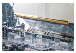
A special design of the MEGA-Speed-Drill-Titan carries out the pre-machining of the main bore of the second lug pack. The tool is led through the first lug pack.
