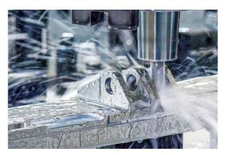
An OptiMill-Titan-HPC is used to machine the gaps between the lugs. ©MAPAL
