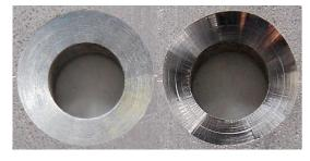
High-quality countersinks for better rivet hole connections: MAPAL countersink (left) compared to a conventional countersink tool (right). ©MAPAL
