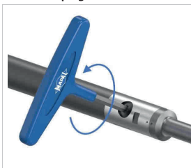
Fig. 19: Undoing clamping stud
