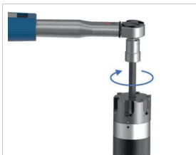
Fig. 12: Tightening threaded spindle to tightening torque
