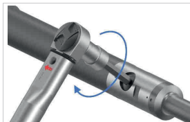
Fig. 16: Tightening clamping stud to tightening torque
