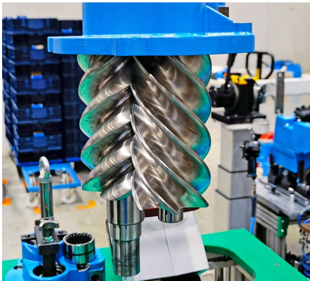
Partially assembled screw compressor assembly, consisting of two rotors and the bearing cover painted blue.
