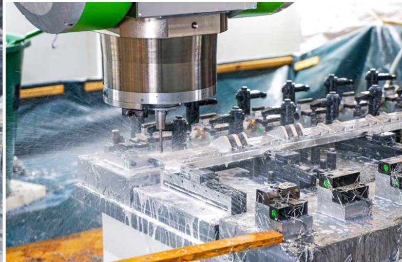
Reaming of an index bore with a fixed reamer from the FixReam range.
