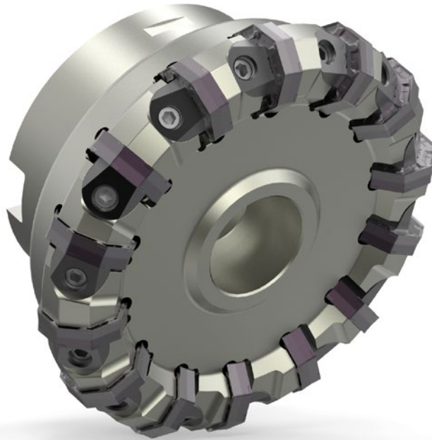
The face milling cutter NeoMill-16-Face is equipped with indexable inserts with 16 cutting edges and machines the connecting surfaces for the manifold flange and exhaust flange.
