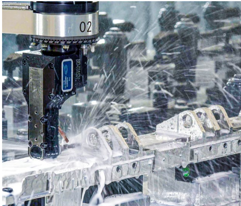
Drilling, countersinking and reverse deburring of a fixing bore with a right-angle drill head.
