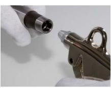
2. Clean the taper, thread and face surface on the replaceable head holder using compressed air
