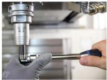
Place your free hand on the replaceable milling head to be able to adjust it sensitively. In this way the tightening torque can be set more accurately.
