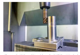
After trochoidal roughing with an OptiMill-Tro-H in the hard material, finishing of the cutting contour of a cutting punch takes place with an OptiMill-3D-CR-Hardened. ©MAPAL
