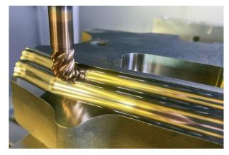
Finishing a mould insert made of powder metallurgical high-speed steel with a hardness of 65 HRC was a great challenge for HaGeForm. With the new OptiMill-3D-CR-Hardened corner radius milling cutter from MAPAL, the machining was accurate down to the  $\mu$ . ©MAPAL
