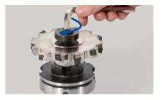
8. Continue to screw the milling cutter clamping screw clockwise with the aid of a hex-wrench and then tighten using a torque wrench (for tightening torque see table "Tightening torque for milling cutter clamping screw").
