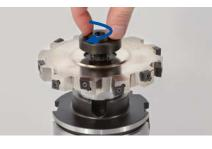
7. Lightly screw the milling cutter clamping screw clockwise into the milling cutter arbor.
