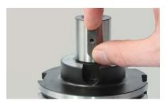
2. Fit the parallel key to the milling cutter arbor.
