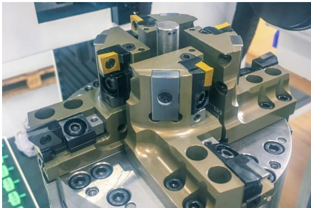
Highly precise setting of the inserts with the UNISSET-V from MAPAL. ©MAPAL
