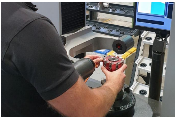
Michael Stockbauer (Application Engineer/Tool Manager MAPAL) setting a 100 mm milling head with PCD milling cartridges. ©MAPAL
